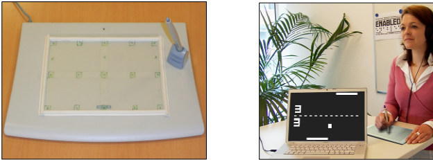
Figure 6 Digitizer tablet provides a frame of reference and absolute positioning
