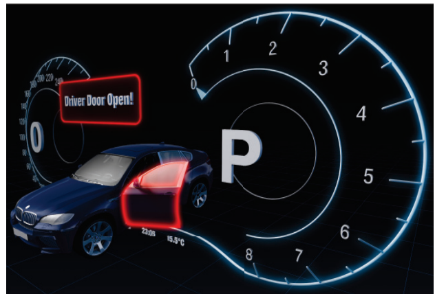
Figure 1: Exemplary illustration of using 3D to highlight important information in the car. While information such as time, temperature, and trip distance remain in the background, a pointer to the open door is shown in the foreground.
