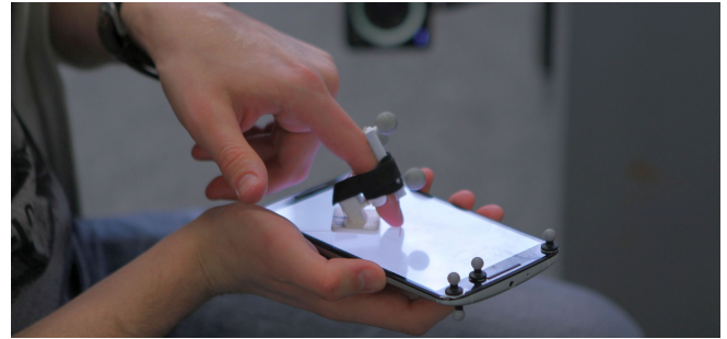
Figure 1. A participants performing a 32.5° pitch and 45° yaw input with the left hand while being equipped with our 3D printed tracking parts.
