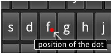
Figure 8. Keyboard that shows a red dot at the position where the user touches the screen after typing an 'f'.
