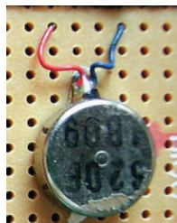
Figure 6: One of the vibrotactile actuators used in the tactile belt.
