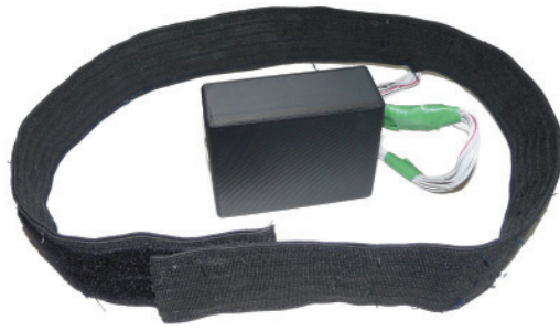
Figure 5: The tactile belt used for the study. The flexible fabrics houses six vibrotactile actuators which equally distribute around the torso if the belt is worn.
