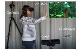
**Figure 1:** User immersed in virtual reality using our TactileDrone system. While tactile feedback is generated by a quadcopter, it is perceived as a hit from a bumblebee.
