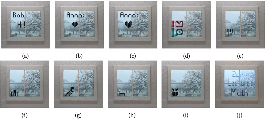
Fig. 6. Demonstrations of the window used as an information display. Messages are shown as text (a) and animated emoticons (b-c). The number of unread messages from different channels is displayed in (d) using icons and edge lighting. Various current activities of a potential communication partner are visualized with icons (e-i). The last picture shows information as shown to passers-by in the context of a lecture hall.
